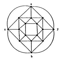
Figure 1: Planar, 5-connected, but not 2-linked graph.
