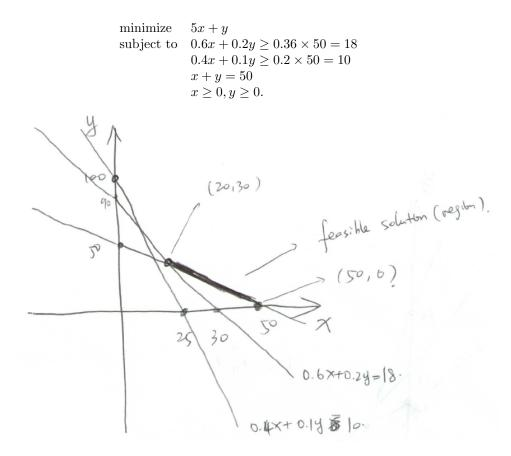
We draw the pictures as above and the feasible region is the line segment connecting (20, 30) and (50, 0). Here x = 20, y = 30 is the solution of 0.6x + 0.2y =
