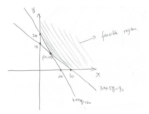
The feasible region is the area in the first quadrant that lies above the two lines. They intersect at the point (10, 12). Therefore we only need to compare the values of the objective function at the points (0, 24), (10, 12) and (30, 0). By calculation, the optimal solution is x = 0, y = 24, meaning that we need to spend all the available hours on the second process. The optimal cost is equal to  $25 \times 0 + 24 \times 20 = 480$ .
