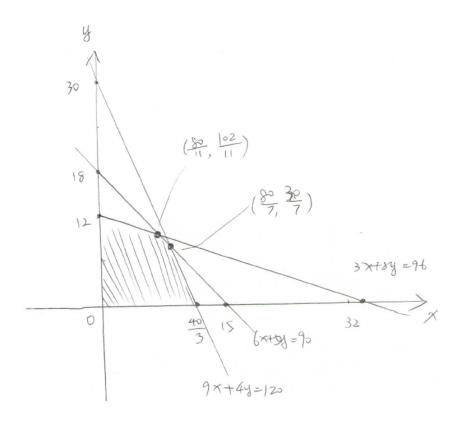
From the picture we know the maximum is achieved among one of the four points: (0, 12), (80/11, 102/11), (80/7, 30/7) and (40/3, 0). Comparing the values of the objective function at these points, we get the optimal solution  $(x, y) = (7\frac{3}{11}, 9\frac{3}{11})$ . (c) (d) To implement such a schedule, we might round up or down the non-
